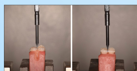
Figure 3. Prepared acrylic test blocks with embedded lower premolars and bonded retainers loaded into the Instron® Testing Machine.
