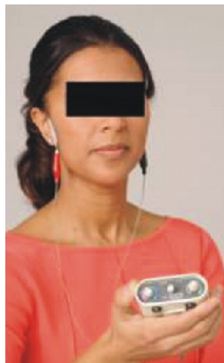
Figure 2. BioTENS,* a ULF TENS unit used for muscle relaxation
