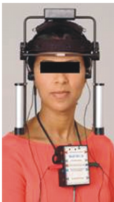
Figure 4. JT-3D* Jaw Tracker used together with EMG to monitor a bite registration
